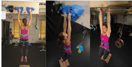
Fig. 2. The RPTC in use, demonstrating the “two arm dead hang (left),” and using weights to tune exercise intensity. In the center, intensity is increased by attaching weights to a harness worn by the athlete. On the right, intensity is decreased by weights acting through a pulley system.
